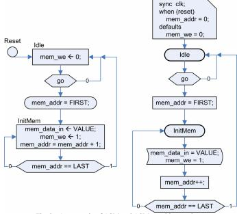
Fig. 3. An example of ASM and ASM++ with assertions.
